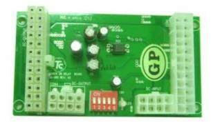
The Delay Board is designed to delay relay switching for applications server system or M/B on delays. If used properly, it will eliminate the need for expensive industrial power switch, which would otherwise be needed to carry out the same task.
